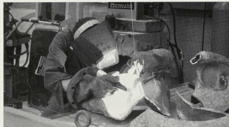
Wearing protective equipment, an artisan welds the cast bronze pieces together.
