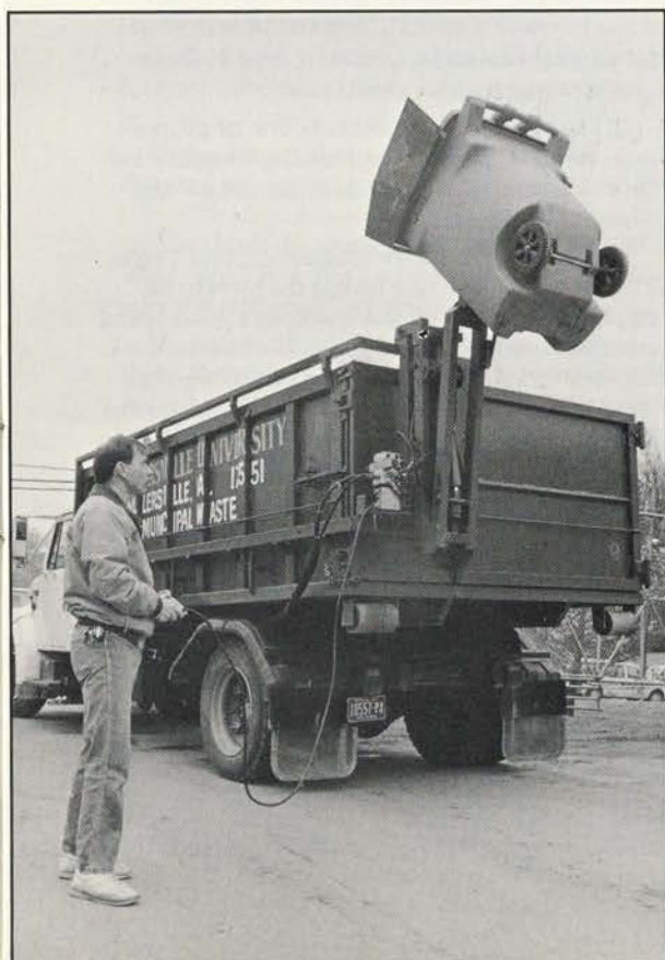
Recycling requires specialized equipment, such as this collector that dumps into separate compartments.
