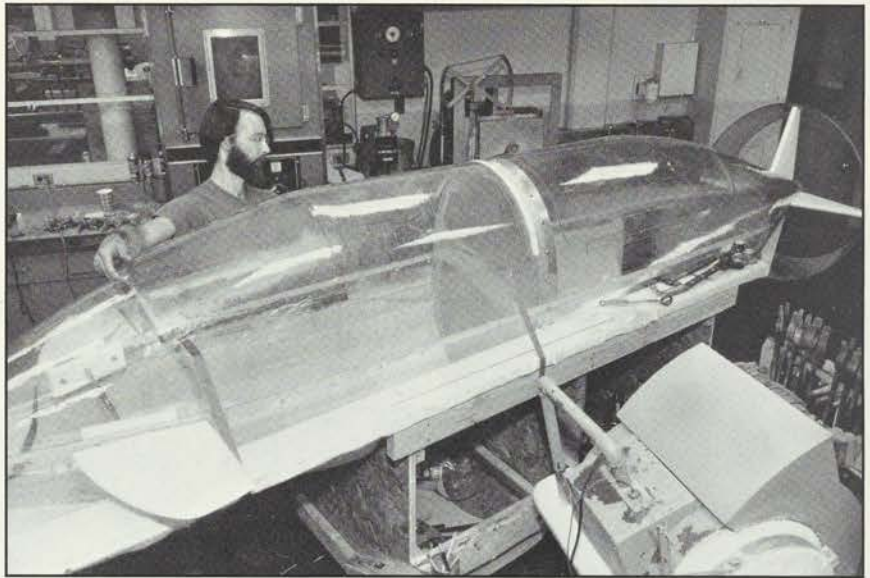
Chris Erickson fits the center hatch into the submarine hull.
